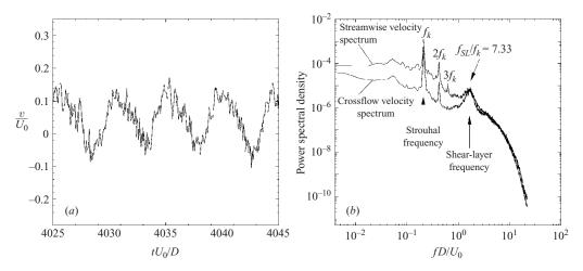
FIGURE 11. Shear-layer instability at Re = 3900. Time history of instantaneous crossflow velocity (only a window of 20 convective time units is shown here) (a) and the velocity power spectra (b) at the point x = 0.54 and y = 0.65 in the shear layer. The power spectrum is obtained by averaging points along the spanwise direction.
