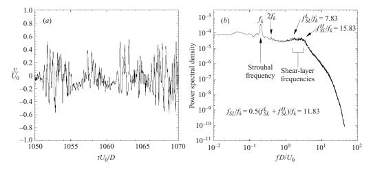
FIGURE 14. Shear-layer instability at  $Re = 10\,000$ . Time history of instantaneous crossflow velocity (only a window of 20 convective time units is shown here) (a) and the power spectra of crossflow velocity (b) at point x = 0.42 and y = 0.55 in the shear layer.
