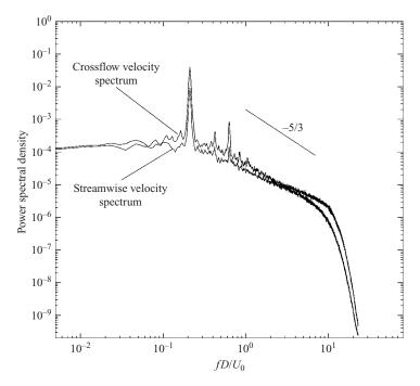
FIGURE 12. Flow spectra downstream of shear layer at Re = 3900. Streamwise and crossflow velocity spectra at the point x = 3.14 and y = 0.40.
