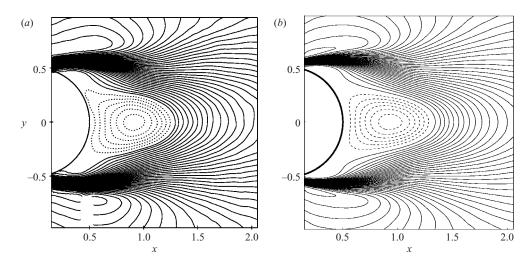
FIGURE 7. Contours of mean streamwise velocity at  $Re = 10\,000$ : (a) PIV; (b) DNS. In both plots,  $u/U_0|_{min} = -0.228$  and  $|\Delta u/U_0| = 0.038$ .
