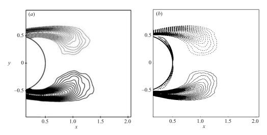
FIGURE 2. Contours of normalized mean spanwise vorticity at  $Re = 10\,000$ : (a) PIV; (b) DNS. In both plots,  $|\bar{\omega}_z D/U_0|_{min} = 1.61$  and  $|\Delta \bar{\omega}_z D/U_0| = 0.32$ .
