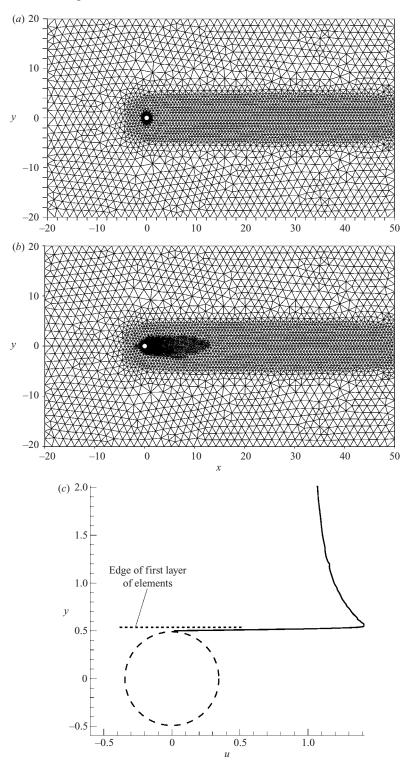
FIGURE 17. Two-dimensional slice of mesh in (x, y)-planes and resolutions for  $Re = 10\,000$  simulations: (a) low-resolution mesh consisting of 6272 triangular spectral elements; (b) high-resolution mesh consisting of 9272 triangular spectral elements; (c) mean streamwise velocity profile along a vertical line crossing the cylinder axis.
