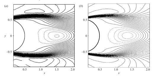
FIGURE 6. Contours of normalized mean streamwise velocity: (a) PIV at Re = 4000; (b) DNS at Re = 3900. In both plots,  $u/U_0|_{min} = -0.252$  and  $|\Delta u/U_0| = 0.063$ .
