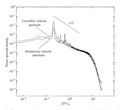
FIGURE 15. Flow spectra downstream of shear layer at  $Re = 10\,000$ . Streamwise and crossflow velocity spectra at the point x = 3.01 and y = 0.38.
