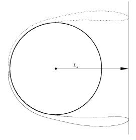
FIGURE 3. Illustration of effective shear layer length  $L_s$ . The mean spanwise vorticity contour in the plot is at a level of 8% of the maximum mean vorticity magnitude along a vertical line crossing the cylinder axis, x = 0.0.
