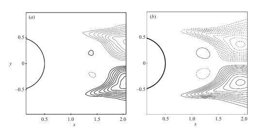
FIGURE 4. Contours of normalized Reynolds stress: (a) PIV at Re = 4000; (b) DNS at Re = 3900. In both plots,  $|\langle u'v' \rangle / U_0^2|_{min} = 0.03$  and  $|\Delta \langle u'v' \rangle / U_0^2| = 0.01$ .
