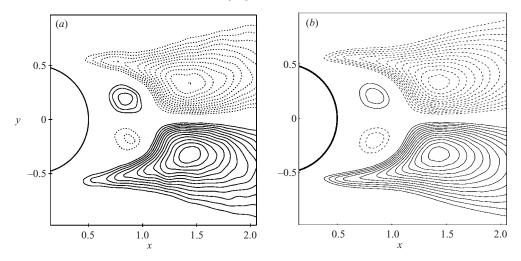
FIGURE 5. Contours of normalized Reynolds stress at  $Re = 10\,000$ : (a) PIV; (b) DNS. In both plots,  $|\langle u'v' \rangle/U_0^2|_{min} = 0.03$  and  $|\Delta \langle u'v' \rangle/U_0^2| = 0.01$ .
