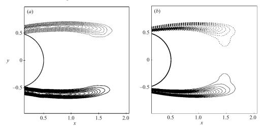
FIGURE 1. Contours of normalized mean spanwise vorticity: (a) PIV at Re = 4000; (b) DNS at Re = 3900. In both plots,  $|\bar{\omega}_z D/U_0|_{min} = 2.58$  and  $|\Delta \bar{\omega}_z D/U_0| = 0.64$ .
